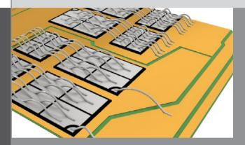
DCB is the traditional technology used for high power applications were currents of 30 A up to several thousand amperes are commonly experienced.
