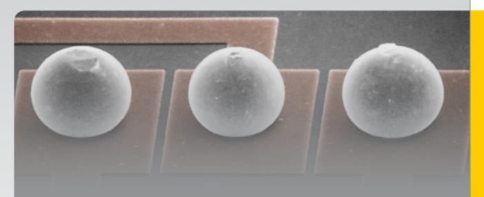
Heraeus has developed Welco-powders for ultra-fine pitch solder paste in various printing applications. The capabilities are ranging from dry film (patented by FCI) to stencil printing. The results of these processes are high quality flip chip or pre-soldered flip chip substrates. These solder powders enable pitches down to  $60 \mu m$ , whereas the printing process represents a more cost effective and flexible bumping method compared to
