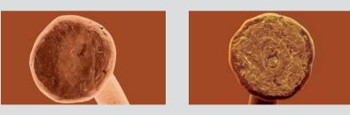
The SEM photographs above show evidence that the intermetallic penetration of the copper ball bond (above left) is significantly less than in the gold ball bond (above right). While this may raise questions as to the integrity of the bond, mid-span pull force tests show an average value of 44.6 grams (3.2 gr Sigma) and shear strength values of 6.5 gr/mi $^{\rho}$ ; values that are, at least, comparable to those obtained with gold wire.
