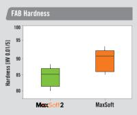
Target FAB: 40 µm Wire Diameter: 0.8 mil EFO Current/Time: 60 mA/265 µs
