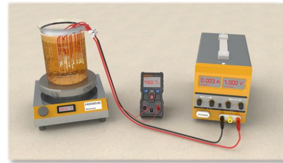
Oil Leak Test
