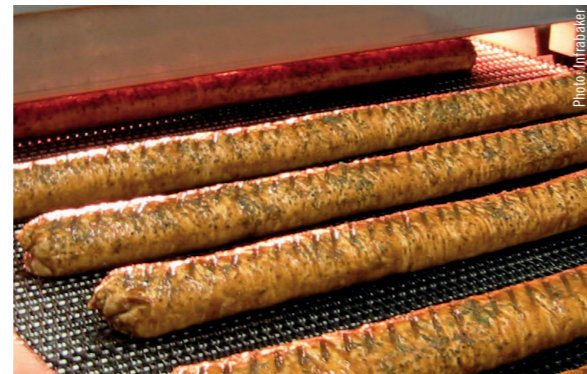
Infrared is used to brown chicken meat for sandwiches
