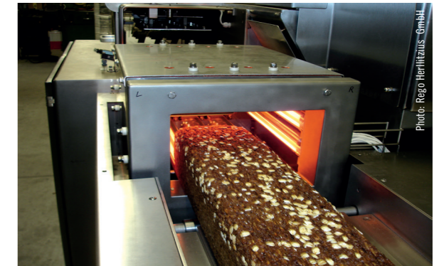
Disinfecting bread before it passes through the bread cutter
