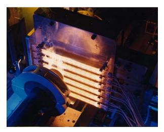
Infrared emitters are arranged in movable plattens that they can be positioned between two pipes. During a few seconds the pipe ends can be weld together.
