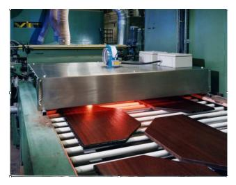
industry away from solvent-based coatings and towards water-based coatings. Initial problems were caused at the point where the UV lacquer was applied over the colour staining. With solvent-based paints, the solvent would "flash off". However, with water-based paints the stain coat is still wet when it reaches the lacquer stage, with the result that the lacquer does not key properly and the correct finish is not achieved.
