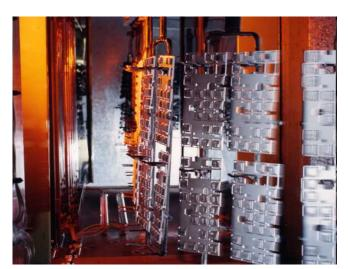
features two 3kW infrared cassettes with medium wave emitters.
