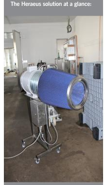
Ozone-free lamps with 254nm UV emission, control unit with 200 W energy consumption and precisely fitting clamping springs.
