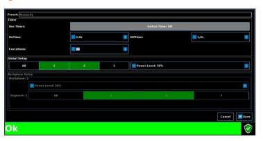
like it does with arc lamp curing systems. In fact, because the UV LED is operating fewer hours, frequent cycling should increase lifetimes. Semray UV LED systems provide the ability to have up to five presets for fast adjustments (dimming, emission width) to meet the process needs of different production runs on the converting or laminating line.
