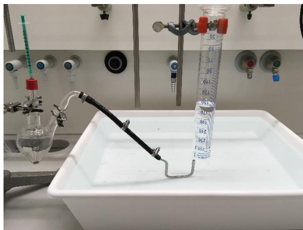
Fig. 1 Laboratory apparatus for \text{H}_2\text{O}_2 decomposition
