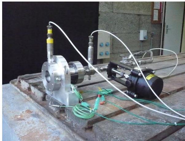
Fig. 9 Monopropellant test facility
